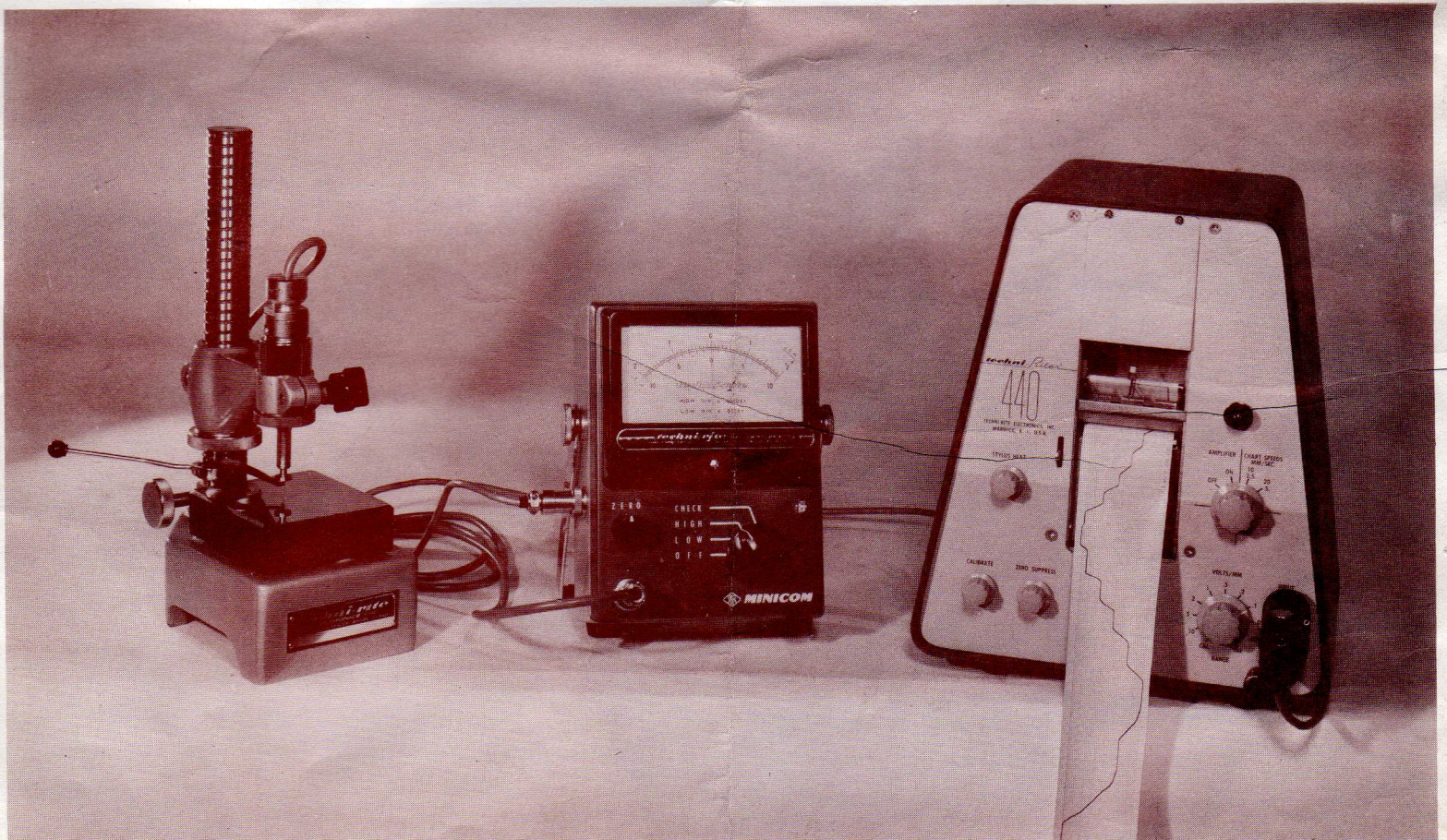
Fig. 5, TR-440 used to record readings from Techni-Rite Minicom
